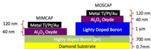
Fig. 1: Schematic of the MIMCAP and MOSCAP stacks
